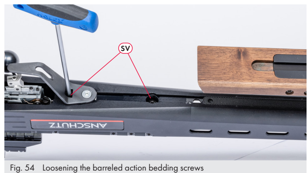
Fig. 54 Loosening the barreled action bedding screws
