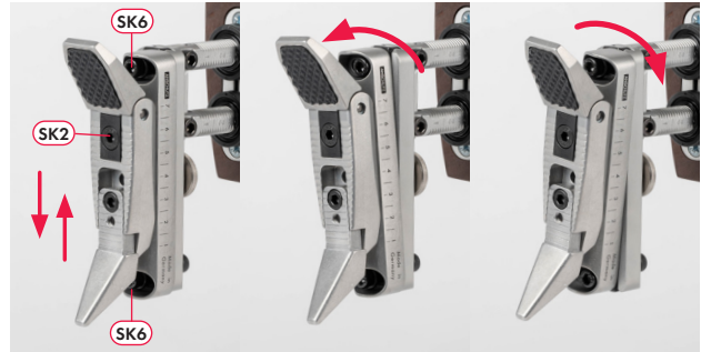
Fig. 90 Tipping the guide rail
