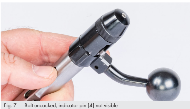
Fig. 7 Bolt uncocked, indicator pin [4] not visible
